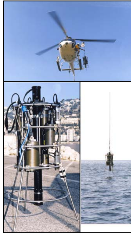
Figure 6. Vertical profiling from a helicopter during the COAST/OOC campaign. Courtesy of M. Babin.
